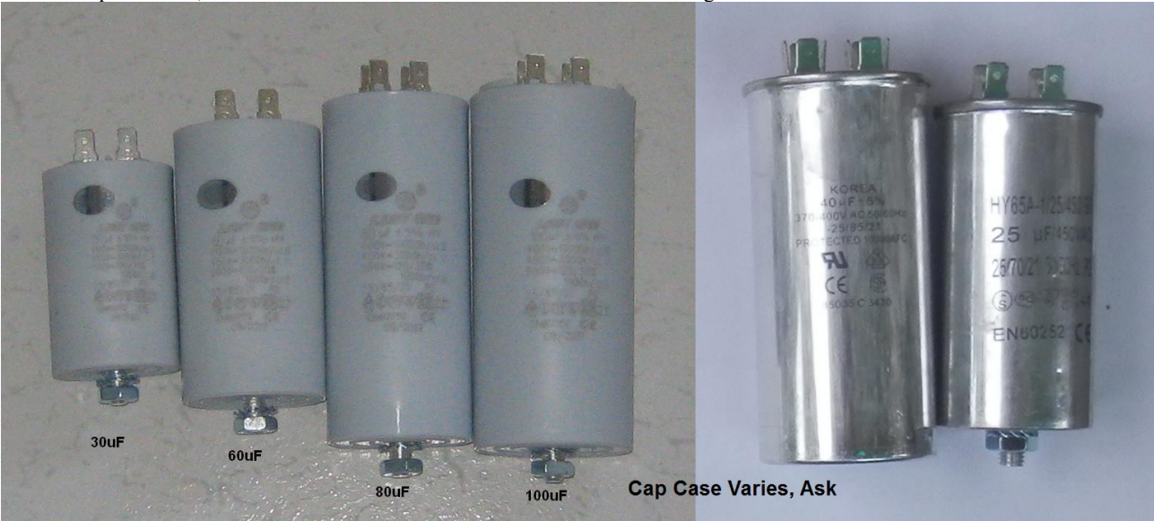
Illustration 3: Some Large Capacitors 25uF to 100uF
